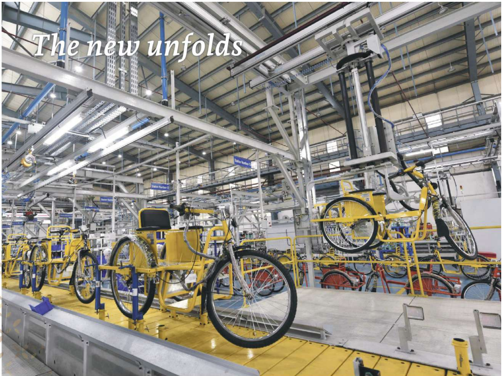
Assembly line with automatic conveyor for assembly of Motorised Tricycle and Wheel chair.
