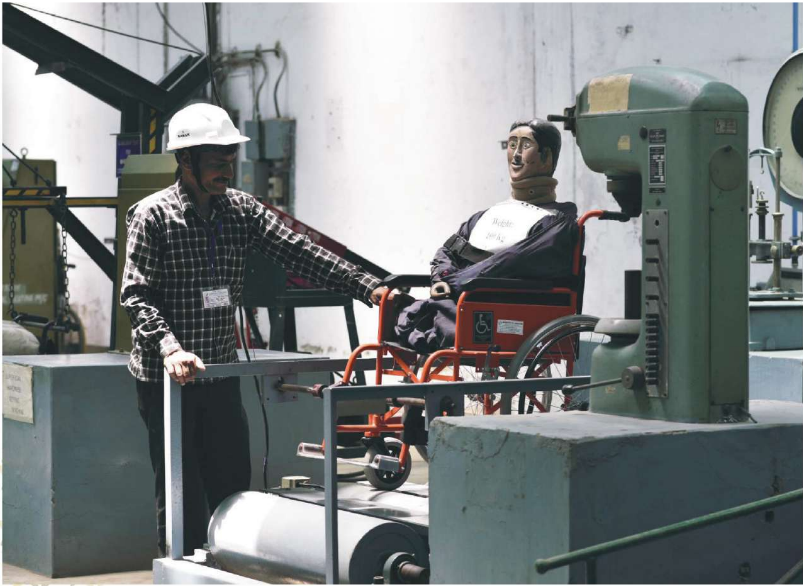
Hazard Running Test for Wheel Chair as per IS : 7454
