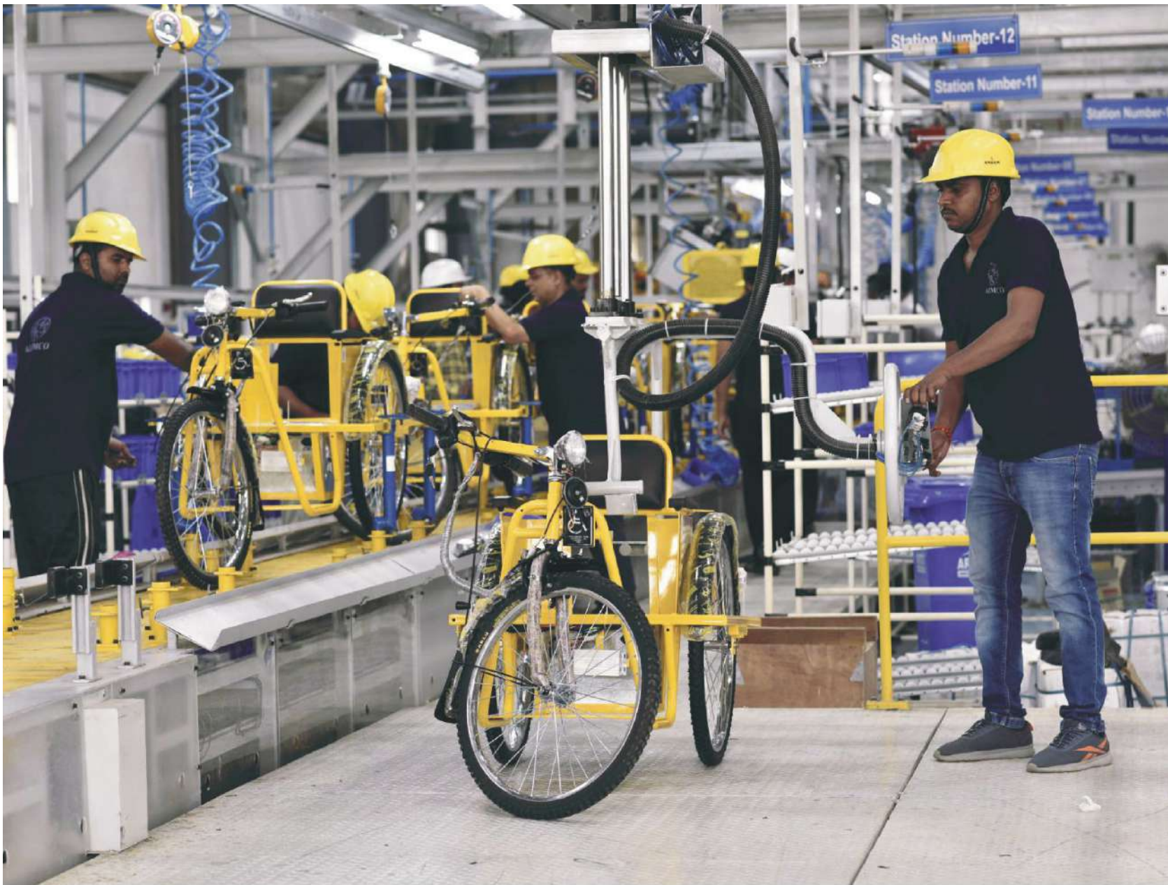
Modern Conveyorized Motorized Tricycles assembly line
