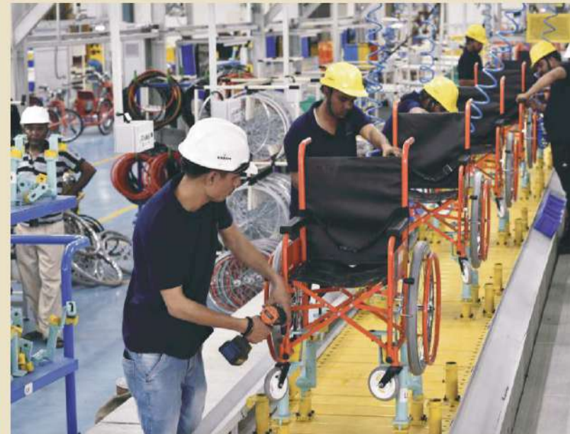
Conveyorized Wheelchair assembly line at WC7.
