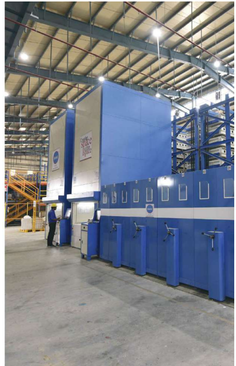
Storage and Retrieval System with Automatic Controls for storage and easy retrieval of tubes, Sheets, tools & bought out parts.
