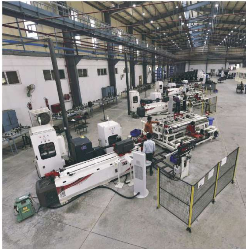
Work Centre - 2 (New Tube and sheet preparation shop) 3 axis & 5 axis bending machines, laser tube and sheet cutting machine.
